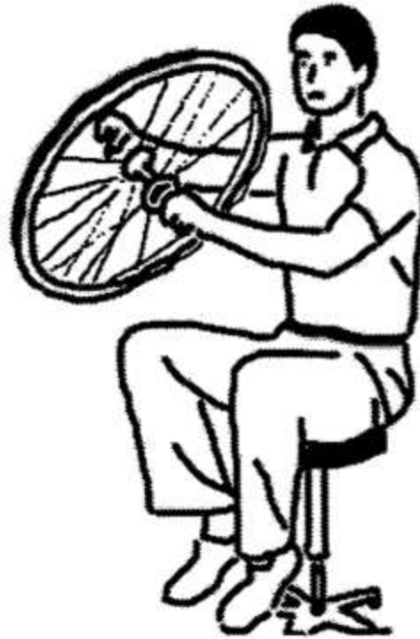
Figure 1.1. While sitting on the rotating chair, the teacher spins the bicycle wheel. When the axis of the wheel is parallel to that of the chair, the latter rotates in the opposite direction of the chair. When the axis of the wheel is perpendicular to that of the chair, no movement should be observed.
